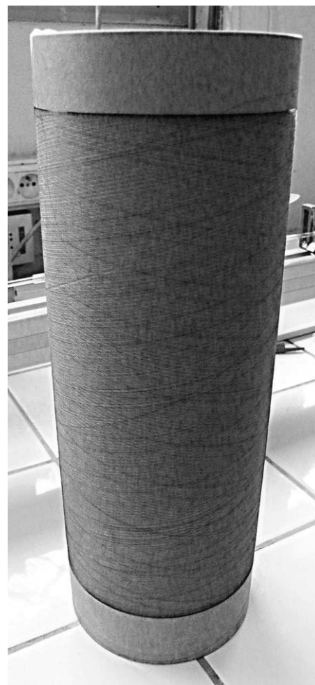
Figure 4 Picture of a several hundred meters long PVA–CNT composite filament on a wheel.
